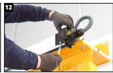
Install a fixed point RG05 next to the end supply (Photos 13 and 14), or two fixed points, one at each side, in the case of intermediate supply (Photo 15). The distance for installing in both cases will be approx. 300mm. Fixed points control expansions and contractions of the line.
