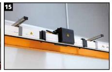
Introduce in the end of the line, or using any housing joint, the collector trolley, by manually pressing the brushes, y taking into account it only has one position: The brush marked as "Earth" has to be located on the side of the PVC profile indicated with black and white stripes, and with an "RG" sticker (Photos 16 and 17).
