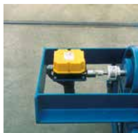
ENCODER + SPINDLE LIMIT SWITCH
